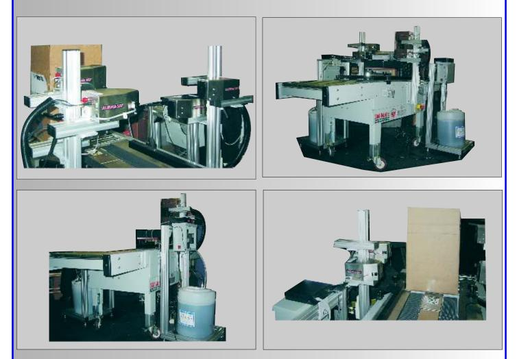
This application uses 5 ajet 101 printers mounted on ajet 101 printers are mounted on opposing sides of the case sealer. Each unit can be controlled individually the 3M case sealer. Two lines of information are using the hand-held input device or can be linked to a printed on one side and two lines on the opposite side. single computer and controlled simultaneously.
