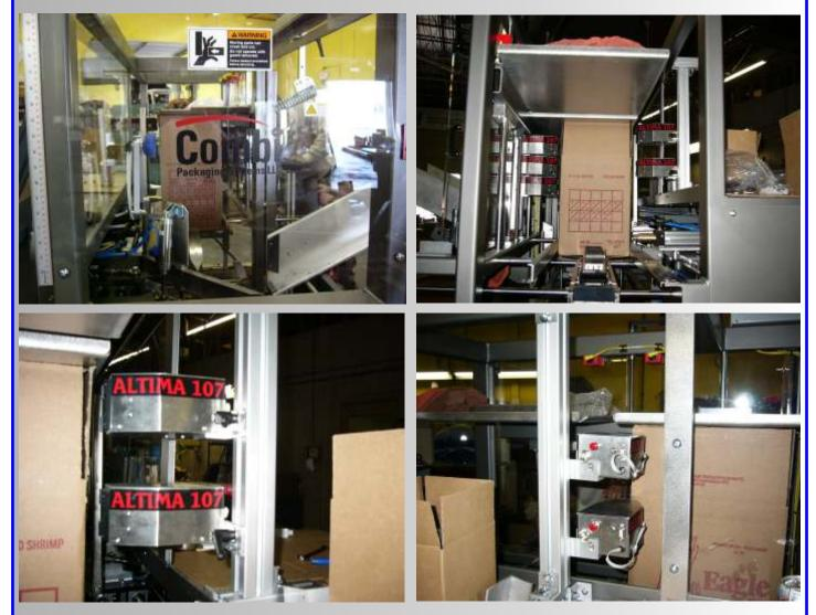
This application uses 5 ajet 101 printers mounted ajet 101 printers are mounted on opposing sides of inside the case handling system. Each unit can be the case handling system. Two lines of information are controlled individually using the hand-held input printed on one side and three lines on the opposite device or can be linked to a single computer and side. Printing is automatic as the case is moved controlled simultaneously.
