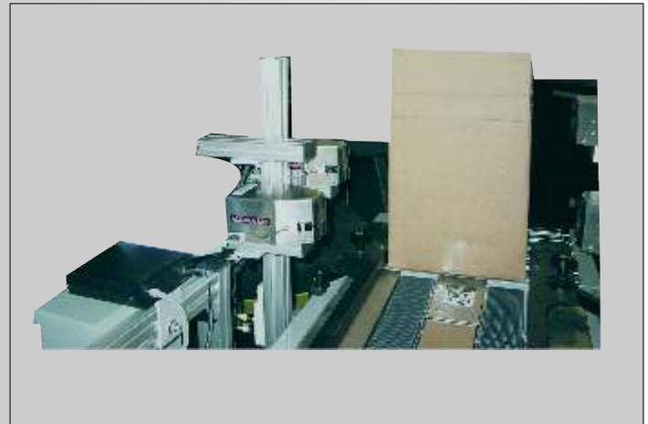
This application uses 5 **ajet 101** printers mounted on the case sealer. Each unit can be controlled individually using the hand-held input device or can be linked to a single computer and controlled simultaneously.
