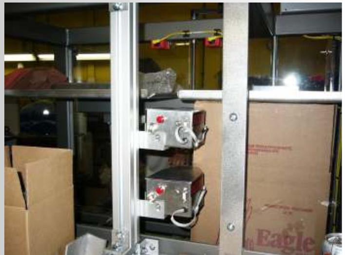
This application uses 5 **ajet 101** printers mounted inside the case handling system. Each unit can be controlled individually using the hand-held input device or can be linked to a single computer and controlled simultaneously.
